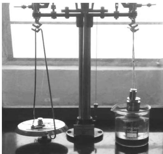
**Figure 1.** Modified analytical balance used for the Mucoadhesion test.
