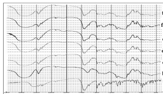
**Figure 2.** FTIR spectra of (a) domperidone; (b) M- $\beta$ -CD and the corresponding drug-carrier molar ratio; (c) physical mixtures 1:1 (PMM1); (d) kneaded 1:1 (KNM1); (e) kneaded 1:2 (KNM2); (f) ultrasonification 1:1 (USM1); (g) ultrasonification 1:2 (USM2).
