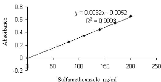
Figure 1. Calibration curve for SMX at 271 nm.
