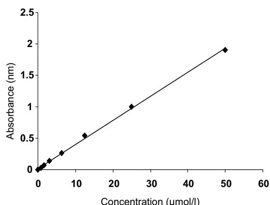
Figure 1. Calibration curve of nitrite at 543 nm (n=?).
