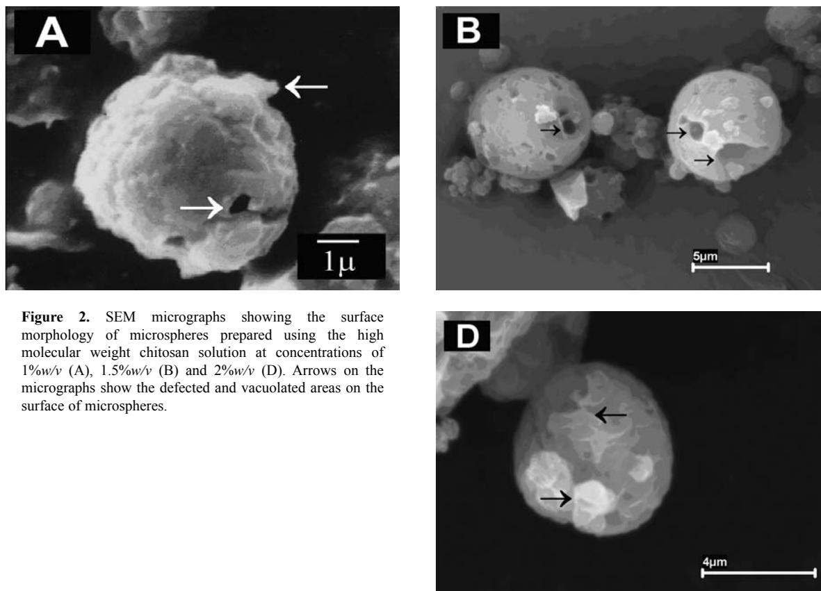
**Figure 2.** SEM micrographs showing the surface morphology of microspheres prepared using the high molecular weight chitosan solution at concentrations of 1%w/v (A), 1.5%w/v (B) and 2%w/v (D). Arrows on the micrographs show the defected and vacuolated areas on the surface of microspheres.
