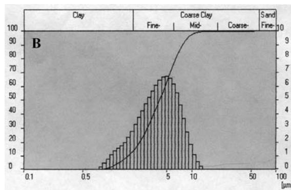
**Figure 3.** Particle size distribution of microspheres prepared using a 1%w/v high molecular weight chitosan solution (n=3).
