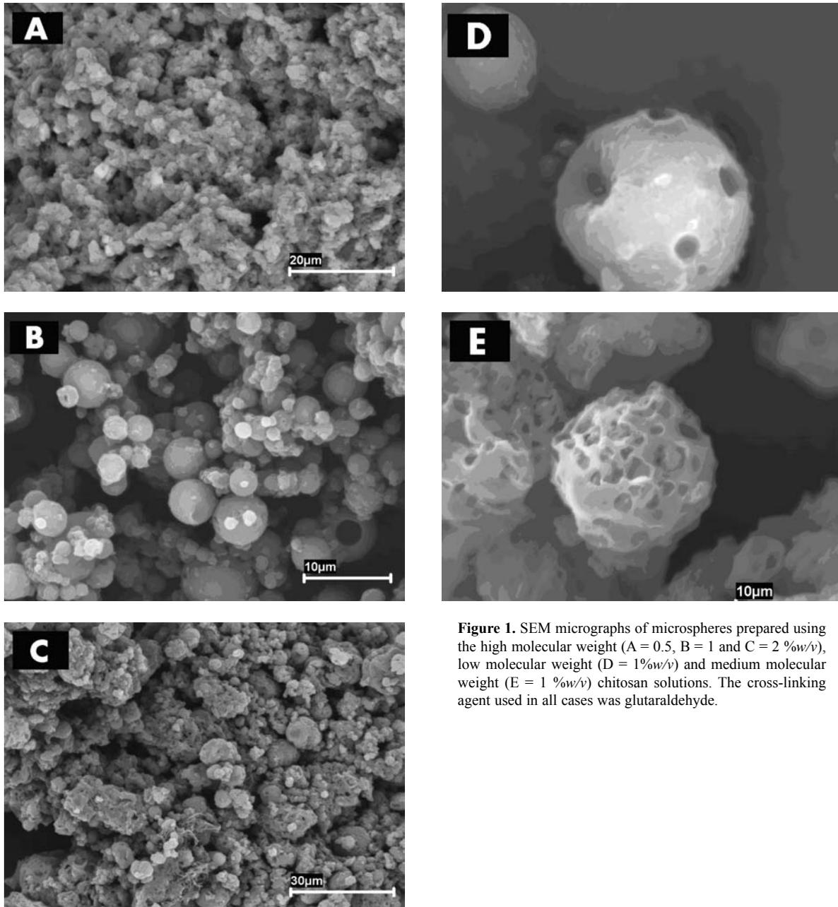
**Figure 1.** SEM micrographs of microspheres prepared using the high molecular weight (A = 0.5, B = 1 and C = 2 %w/v), low molecular weight (D = 1%w/v) and medium molecular weight (E = 1 %w/v) chitosan solutions. The cross-linking agent used in all cases was glutaraldehyde.
