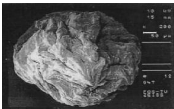
Figure 1. Scanning electron microscopy image of gelatin microspheres.
