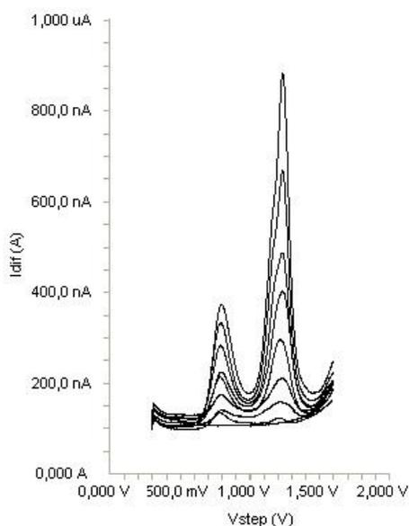
**Figure 5.** SWV voltammograms obtained for the determination in supporting electrolyte (blank, 1.5, 2.5, 5, 7.5, 10, 12.5, 15 and 17.5  $\mu\text{g mL}^{-1}$ ).
