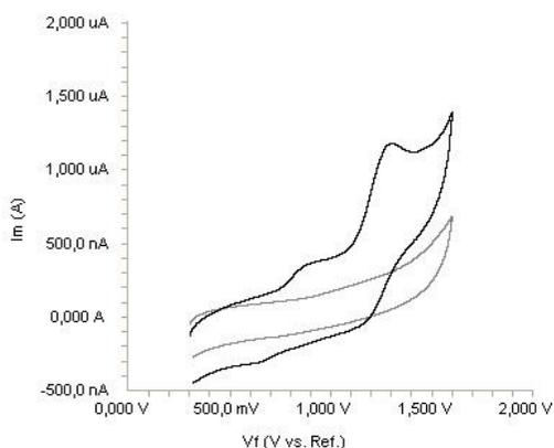
**Figure 2.** Cyclic voltammogram for the oxidation of 20  $\mu\text{g mL}^{-1}$  diclofenac in acetonitrile containing 0.1 M TBAClO<sub>4</sub> at Pt disk electrode, scan rate: 0.2 V s<sup>-1</sup>.
