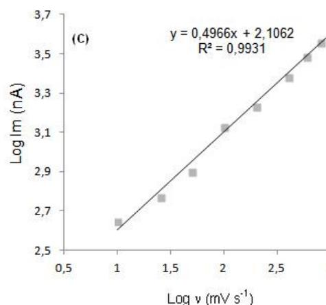
**Figure 4.** Dependence of peak current on the scan rate (20  $\mu\text{g mL}^{-1}$ ).
