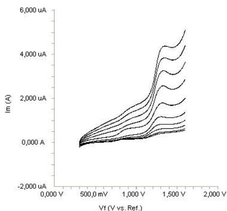
**Figure 3.** Linear sweep voltammograms for the oxidation of 20  $\mu\text{g mL}^{-1}$  diclofenac in acetonitrile containing 0.1 M TBAClO<sub>4</sub> as a function of scan rate.
