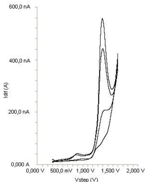
**Figure 6.** SWV voltammograms obtained for the determination in spiked serum (blank, 5, 10 and 15  $\mu\text{g mL}^{-1}$ ).
