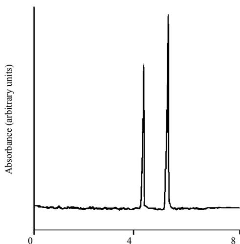
**Figure 4.** Separation of aciclovir and guanine under CZE conditions using a buffer of higher pH. Conditions: capillary 720 mm (500 nm to detector), buffer sodium tetraborate 20 mM, pH=9.8, voltage 25 kV, wavelength 254 nm, temperature(25°C)
