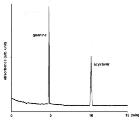
Figure 2. Electropherogram showing separation of aciclovir and guanine in low pH buffer. Conditions: capillary 720 mm (500 nm to detector), buffer sodium citrate 20 mM pH=2.5, voltage 30kV, wavelength 254 nm, temperature(25°C)
