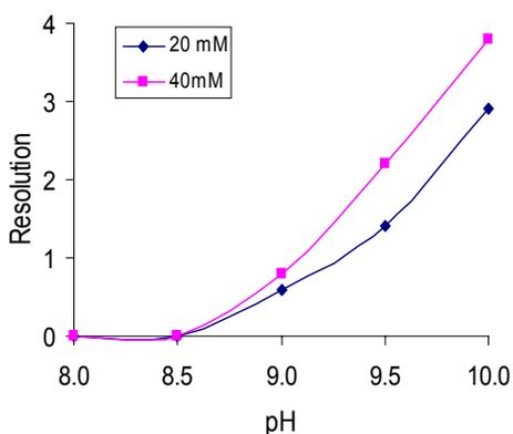
**Figure 3.** Resolution of aciclovir and guanine at two levels of the buffer concentration against pH of the buffer (conditions as described in Figure 4).
