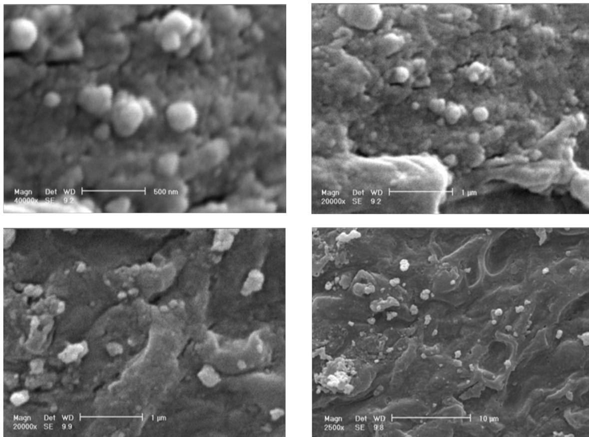
**Figure 8.** SEM micrographs of silver nanoparticles produced by the reaction of 1 mM AgNO<sub>3</sub> solution with *F. oxysporum*.
