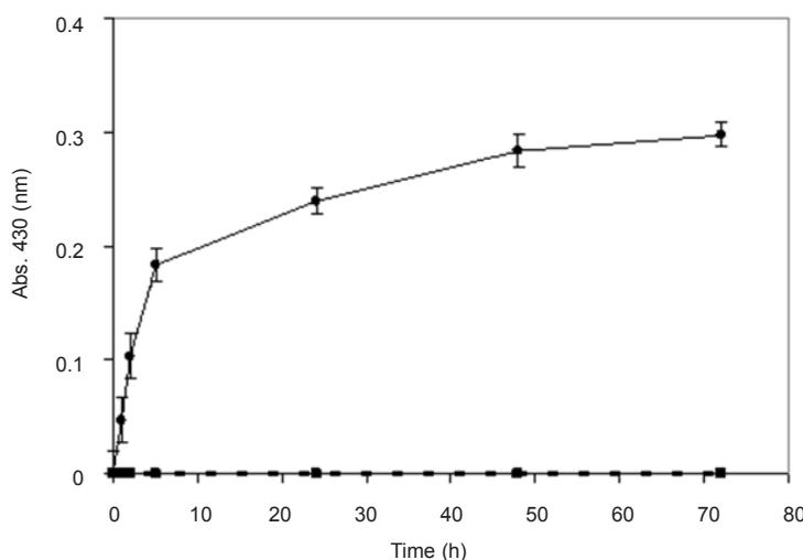
**Figure 3.** Time course of biotransformation of  $\text{AgNO}_3$  using non-boiled (●) and boiled (○) biomass. The spectrum was obtained at different time points after the start of  $\text{AgNO}_3$  (1 mM) reduction using *F. oxysporum* previously induced with  $\text{AgNO}_3$  (0.1 mM) ( $n$ -value= 3).
