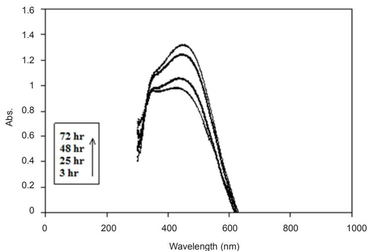
**Figure 2.** UV/Vis absorption spectrum of the produced colloidal Ag. The spectrum was obtained at different time points after the start of  $\text{AgNO}_3$  (1 mM) reduction using *F. oxysporum* previously induced with  $\text{AgNO}_3$  (0.1 mM).
