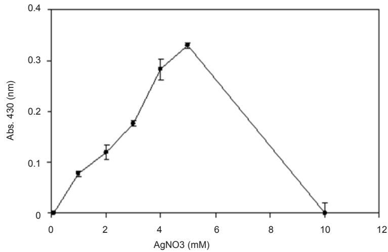
**Figure 6.** Effect of different concentrations of the substrate- Absorption spectra of maximum production of silver nanoparticles against various concentrations of AgNO<sub>3</sub> (0.1, 1, 2, 3, 4, 5, and 10 mM) was read and recorded ( $n$ -value = 3).
